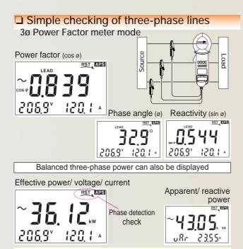
The 3286's three-phase power measurement calculates and displays the power values for a sine wave input at 50/60 Hz, assuming it is balanced and there is no distortion. Accurate measurement is not possible on a three-phase line if it is not balanced, for example when controlled by an inverter or thyristor.
